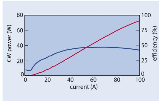
**Fig. 5.** Alfalight’s SE-DFB laser can produce a continuous-wave output of 73 W, which is a record for a single chip. The efficiency of this source is 50%.
