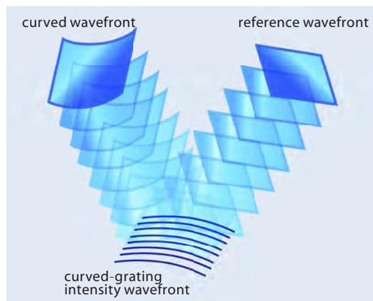
**Fig. 3.** Curved gratings that feature in the SE-DFB laser are formed by interference of a reference plane wavefront and curved wavefront. The reference wavefront comes from a collimated laser beam and the curved wavefront is generated by the collimated beam exiting the phase plate surface.
