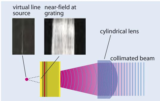
**Fig. 4.** The SE-DFB laser produces a lateral beam with a cylindrical wavefront that appears to emanate from a narrow virtual line source behind the grating surface. The wide stripe is an image captured at the grating surface and the narrow stripe is a virtual line source formed at the focus behind the chip.
